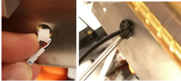
Make sure the cable is pulled over the cross bracket inside the print unit.
