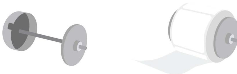
Orient the label roll as shown. Then install it on the roll holder. Make sure the side of the roll is pressed flush against the wide flange.
