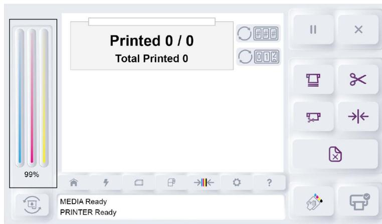
The ink level will be displayed using visual CMY bars. The ink level is also displayed as a percentage under the bars. After installing the new ink cartridge, the ink level will be shown as full (100%).
