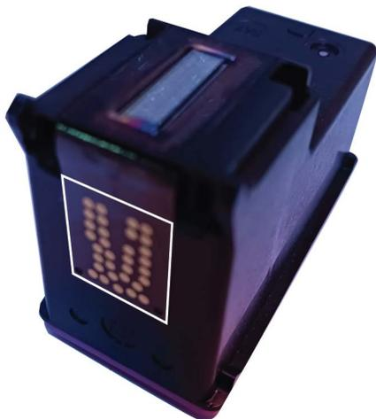
6. Hold the ink cartridge so that the copper strip is on the bottom and facing the printer. Slide the ink cartridge into the cradle as shown.
