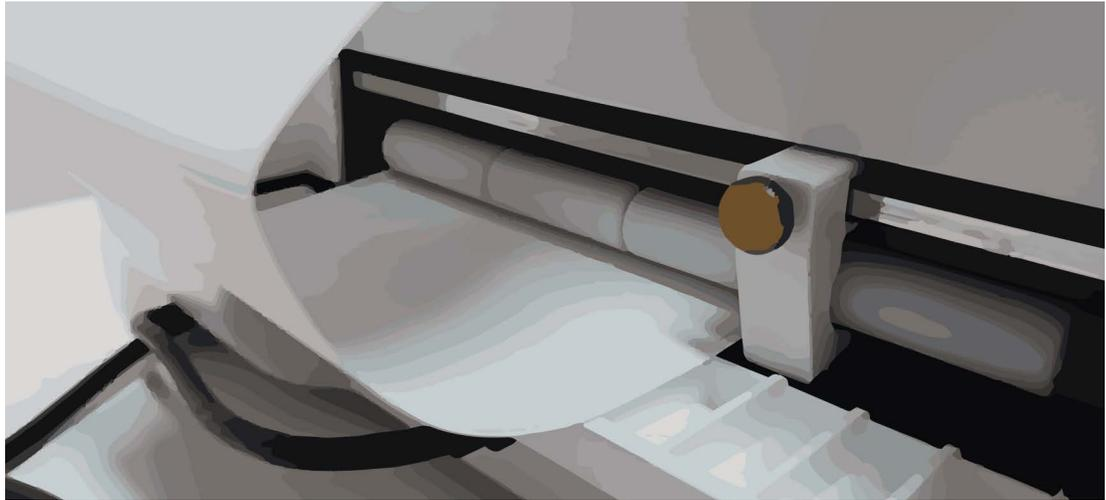
Unroll a small amount of labels. Then feed the first label of the roll into the media entry slot. Make sure the edge of the media is against the left side of the slot.
