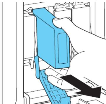
4. Take out the ink cartridges from the package. Then remove the packing materials.
