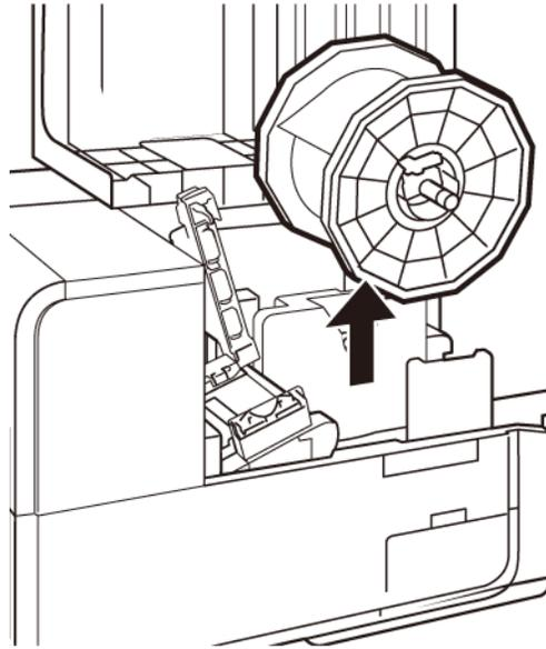
6. Release the holder stopper screw, and remove the holder stopper from the roll holder.
