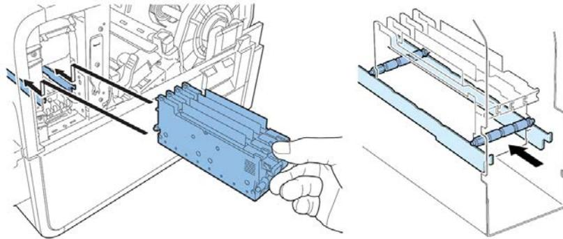
If printhead is insufficiently inserted, the lower printhead release lever cannot be closed. To confirm printhead is in the correct position, see if the end of printhead grip and the edge of the inner metal plate are in the same plane as shown in the figure.
