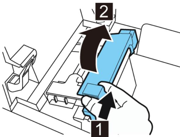
9. Open the transport guide (right), and slide it rightward until it stops.
