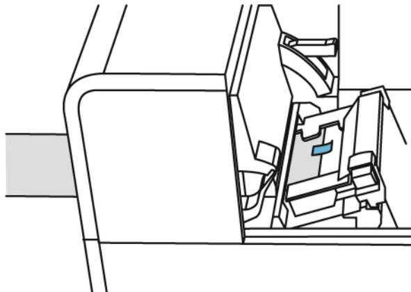
3. Push the lever of the paper guide to open the guide.
