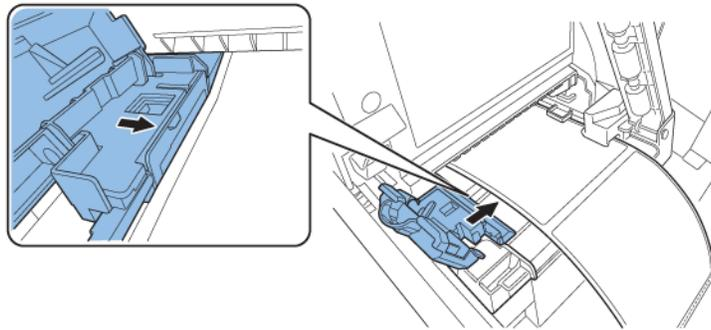
**Note:** Do not press the transport guide (right) strongly against the media edge. A paper jam can result.
