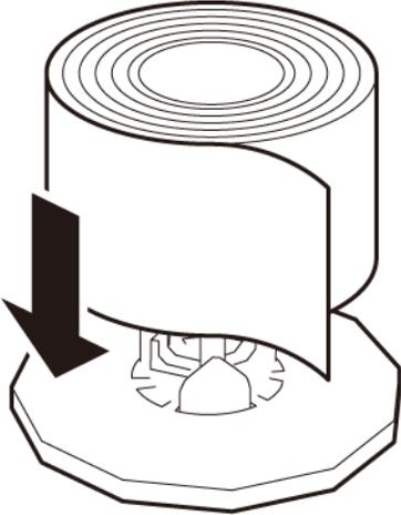
5. Insert the holder stopper until it stops, and tighten the holder stopper screw.
