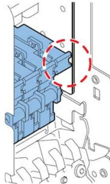
12. Mount the blade cleaner in the printer. The blade cleaner (B) rests on the alignment slots used by the printhead (A).
