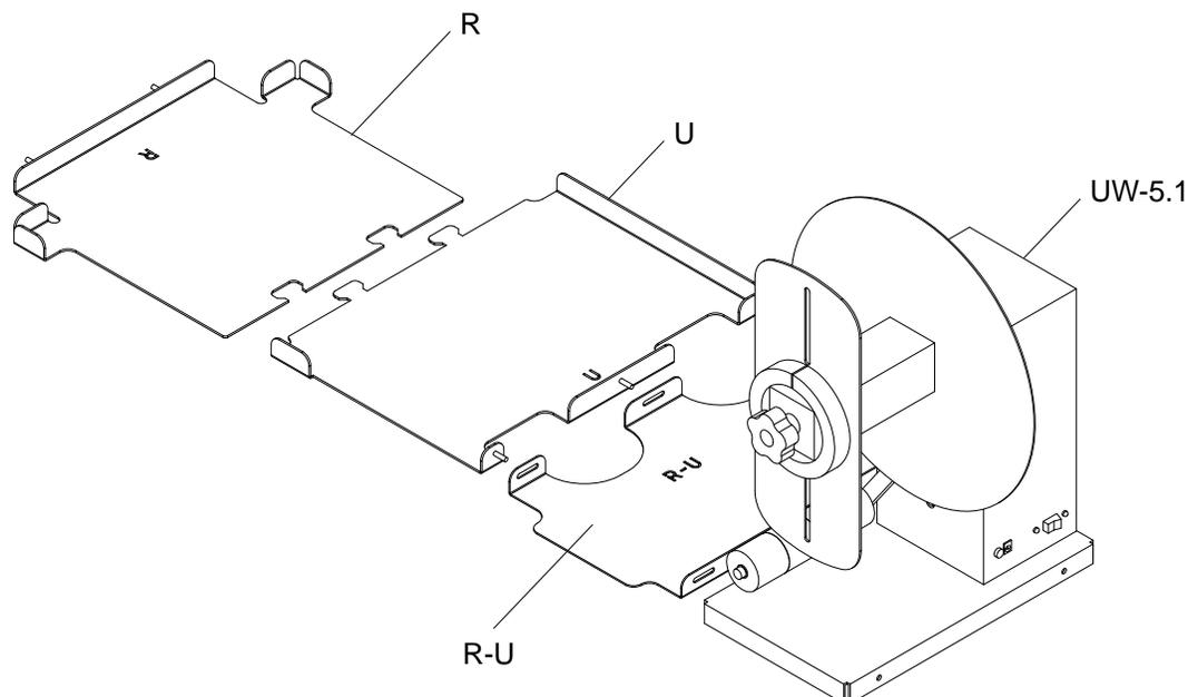
3. Insert the tabs from bracket U into the slots on bracket R. These two brackets will later be used to position the printer.
