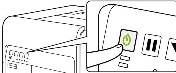
The Power LED blinks at long intervals, and then the printer is turned off.
