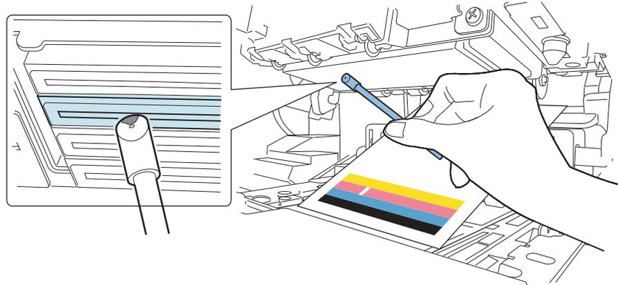
**Caution:** Do not touch cut section of cleaning stick on face of Printhead. Do not touch Printhead surface with your hand.
