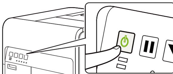
Cleaning is performed and the printer becomes ready for printing. When the printer is in the Online mode, the STATUS LED stays lit.
