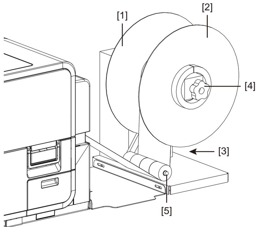
2. Turn the unwinder mandrel adjustment knob [4] counterclockwise to loosen the mandrel.
