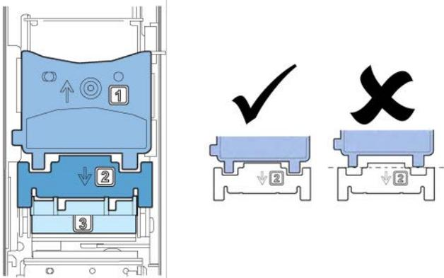
If any numbers (1), (2), or (3) are invisible, the printhead release lever (1, 2) has not been closed or the blade cleaner (3) has not been mounted. Review work procedure.
