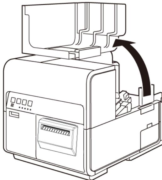
7. Remove the roll holder from the printer. The roll holder is unnecessary when using the unwinder.
