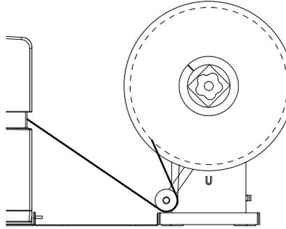
As the dancer arm is lifted, the mandrel will unwind and feed media as needed. Do not turn the unwinder mandrel by hand to advance the media. If you need to advance the media, lift the dancer arm slightly.
