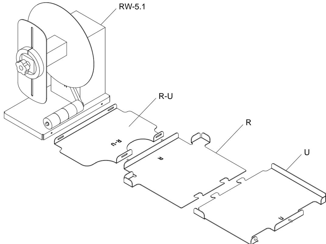
3. Insert the tabs from bracket U into the slots on bracket R. These two brackets will later be used to position the printer.
