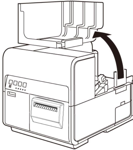
3. Push the lever of the paper guide to open the guide.
