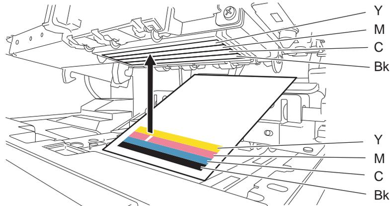
8. Touch the tip of cleaning stick on nozzles that have non discharge, and then hold for five seconds to absorb ink.
