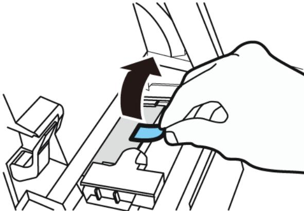
5. While pushing the pinch roller release lever, pull out media through the delivery slot.
