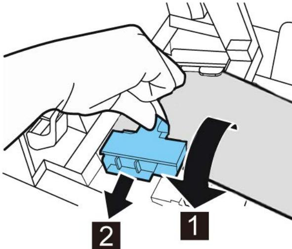
4. While pressing the pinch roller release lever, pull out the media.
