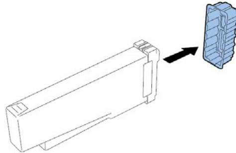
Do not touch the ink outlet and terminal to prevent soiling of the surrounding work area, damage to the ink cartridge, and poor printing. Never drop or apply excessive force to an ink cartridge.
