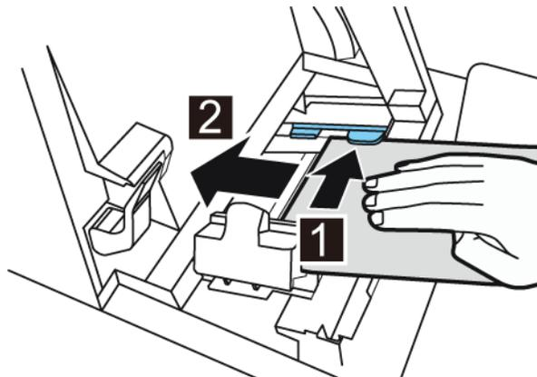
Media at the roller in the feeder slot is automatically pulled in slightly.
