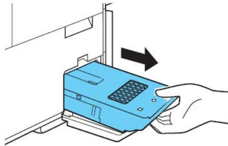
When removing the maintenance cartridge full of ink, take care not to incline or drop it. The spilled or scattered ink may stain the floor or clothing.
