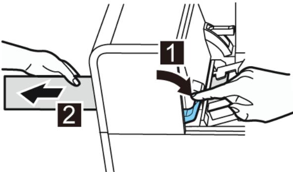
6. Remove the empty roll holder. Remove the empty roll core from the roll holder.
