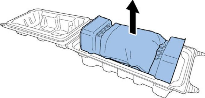
**Caution:** Do not touch the printhead face. An ink injection problem can occur. Hold the printhead only by the end tab.
