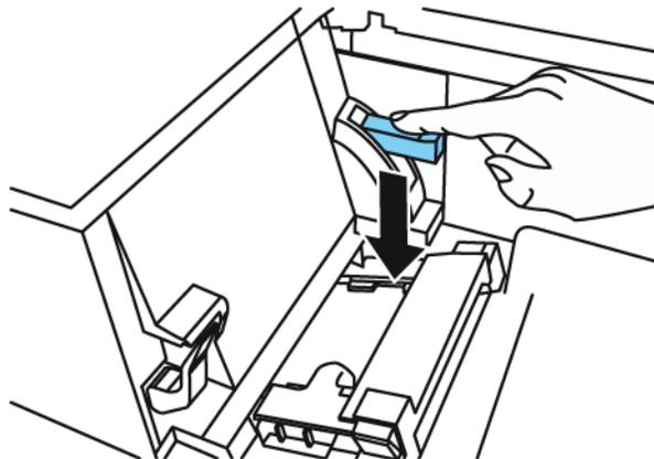
4. While pushing the pinch roller release lever, pull out paper in the direction opposite to the transport direction.
