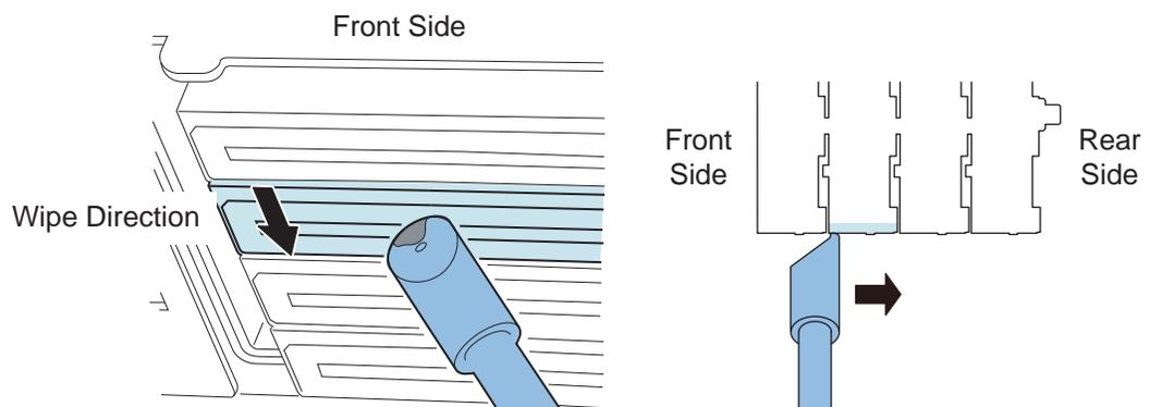
**Caution:** Touch cleaning stick to the face of Printhead so tip of cleaning stick bends lightly.
