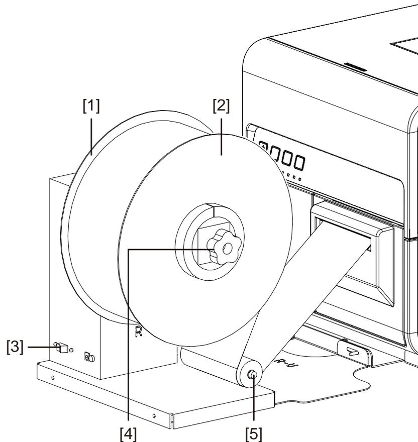
2. Turn the rewinder mandrel adjustment knob [4] counterclockwise to loosen the mandrel.
