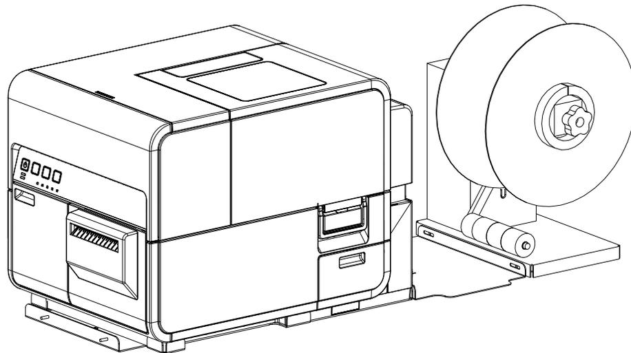
10. Plug the power jack into the power slot on the unwinder. Insert the power plug into an AC power receptacle.
