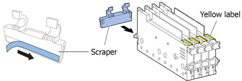
Handle the scraper with care, and do not touch the blue area along the bottom of the scraper.
