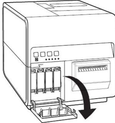
2. Open the ink cartridge lever while pushing it downward.
