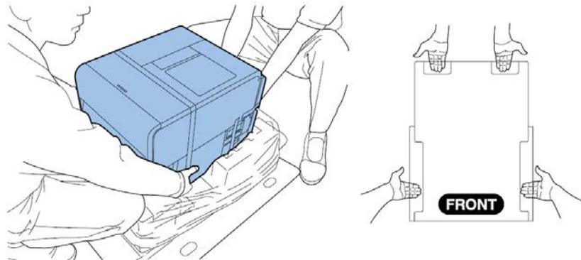
**Note:** The printer weighs about 53 pounds (24 kilograms). Two persons are required to lift the printer. Two persons standing at the front and back of the printer respectively must lift the printer by holding it with their hands under the bottom handles (two at the front, one at the left, and one at the right). Attempting to lift the printer in an improper position can result in the printer falling or injury.
