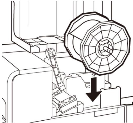
The flanges and corresponding installation points in the printer are color coded. Orient the roll holder so the black flange matches the black installation point, and the gray flange matches the gray installation point.
