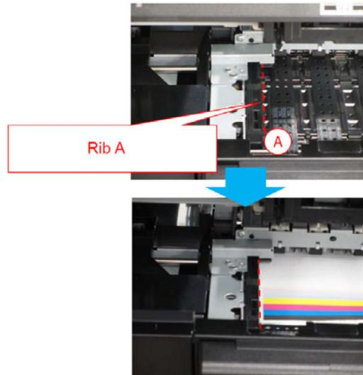
7. Find the void on the printed label and take note of where and which printheads are affected by non-discharging nozzles.
