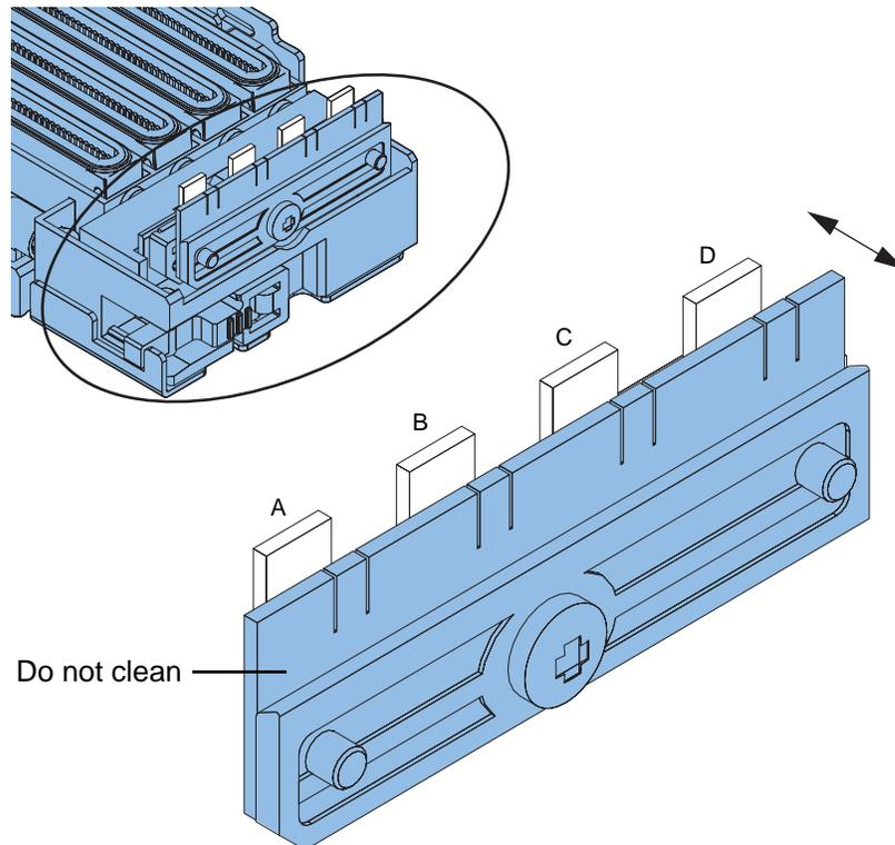
4. After wiping the top surface, wipe the face surface of the blade (A, B, C, and D). Then wipe the back surface of this blade.
