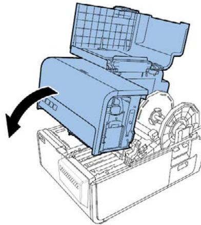
5. Remove the print module cover. Then open the upper printhead release lever and lower printhead release lever.
