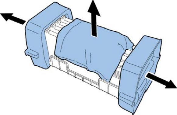
8. Remove the caps from the printhead ink supply ports.
