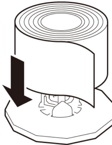
3. Insert the holder stopper until it stops, and tighten the holder stopper screw.
