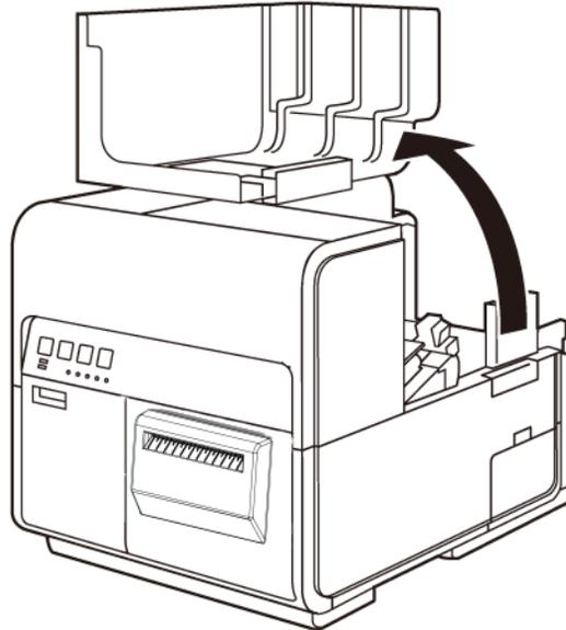
2. Push down the upper unit release lever and then open the upper unit.
