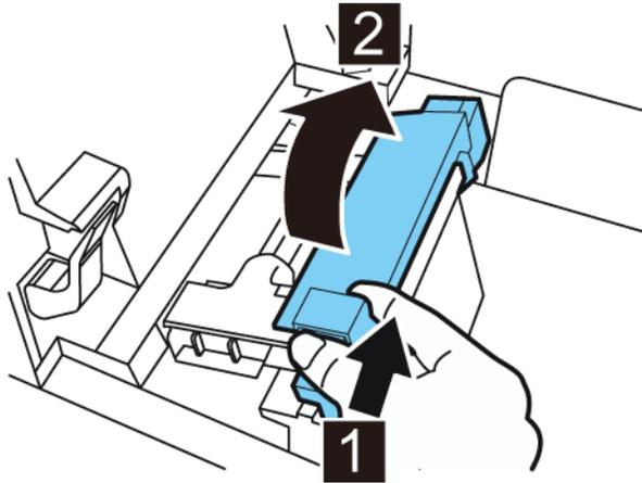
4. Open the transport guide (right), and slide it rightward until it stops.
