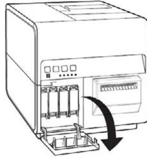
2. Open the ink cartridge lever for each color while pushing it downward.
