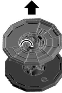
2. Load roll media on the roll holder with it oriented as shown such that the bottom of the roll touches the roll holder surface with no clearance.
