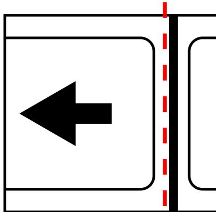
7. Insert media along the left-side guide under the transport guide (left) until it stops at the roller in the feeder slot.
